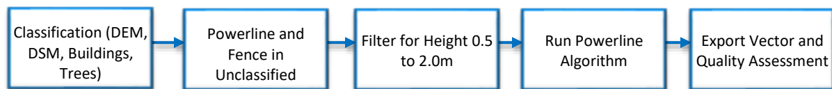
Figure 4-3: Workflow for Powerline Extraction Algorithm
