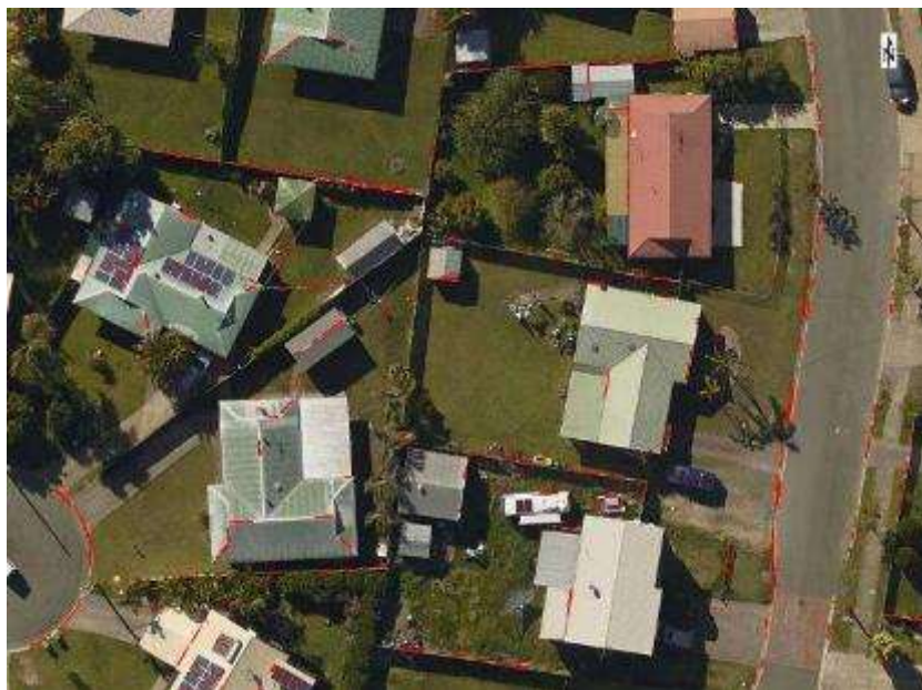
Figure 4-13: Fence-line extracted using image segmentation with false positives and omissions
