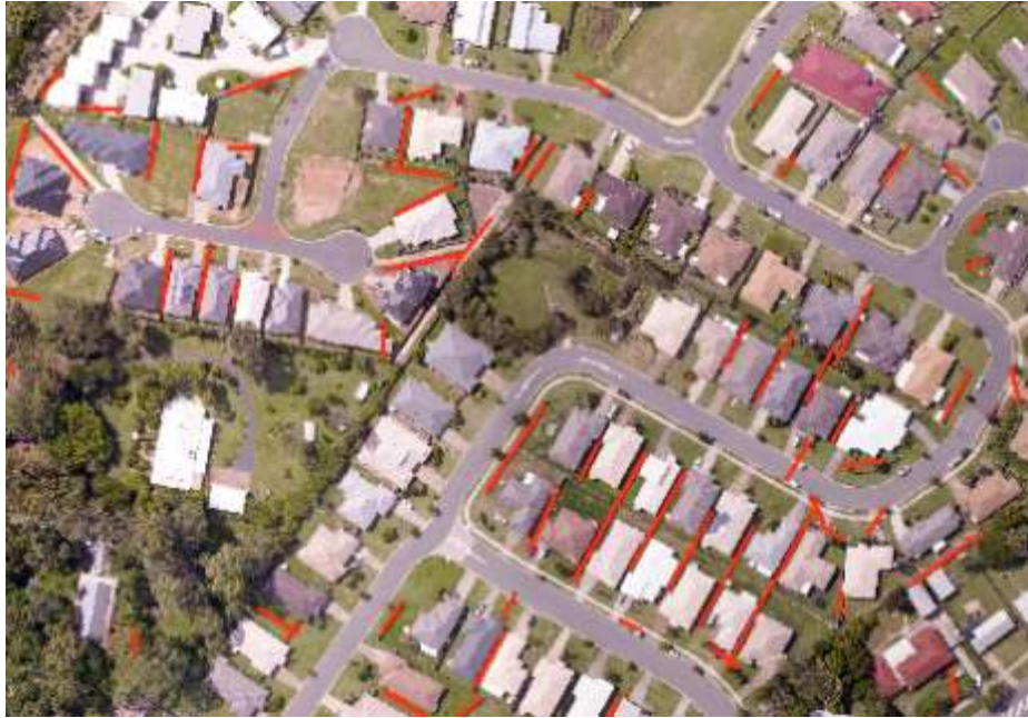
Figure 5-25: Fence-lines extracted from low resolution Lidar for (Top) Horizontal and (Middle) Vertical directions of flight; and (Bottom) the combined Lidar results
