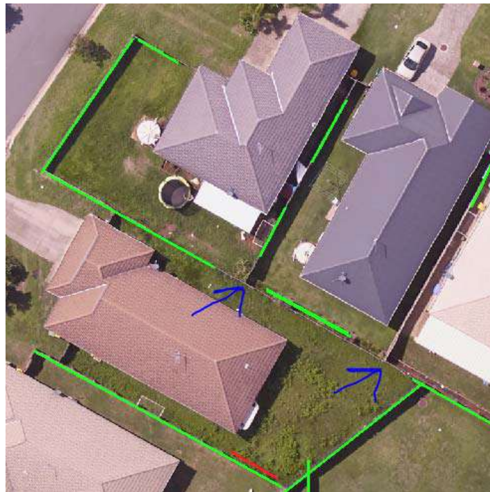
Figure 6-4: Missing fence intersection lines because of circular coverage reduction of point cluster by the tree removal algorithm
