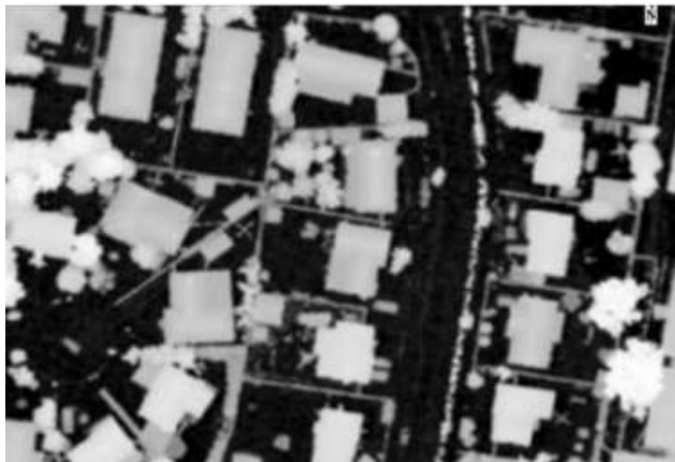
Figure 4-6: Surface difference from DSM-DEM derived from Lidar
