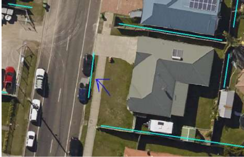
Figure 6-6: An example of parked cars being misclassified as a fence line is shown here, (blue arrow)
