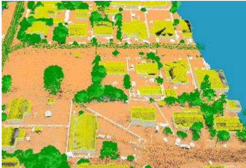
Figure 4-4: Points in white represent fence but other unclassified points are classes as fence as well
