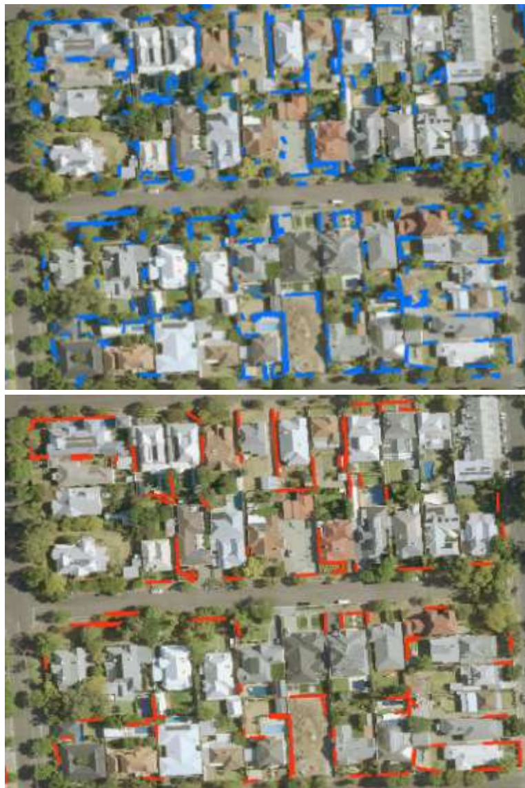
Figure 5-15: Adelaide Lidar processing (Top) Unfiltered fence-lines (Bottom) Filtered lines
