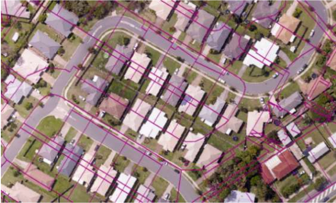
Figure 5-18: Simulated distortion of the digital cadastre
