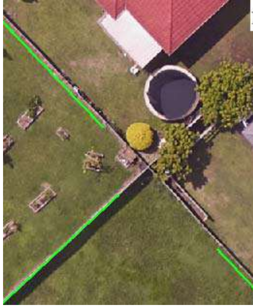
Figure 6-3: An example of fence line segments missed due to vegetation
