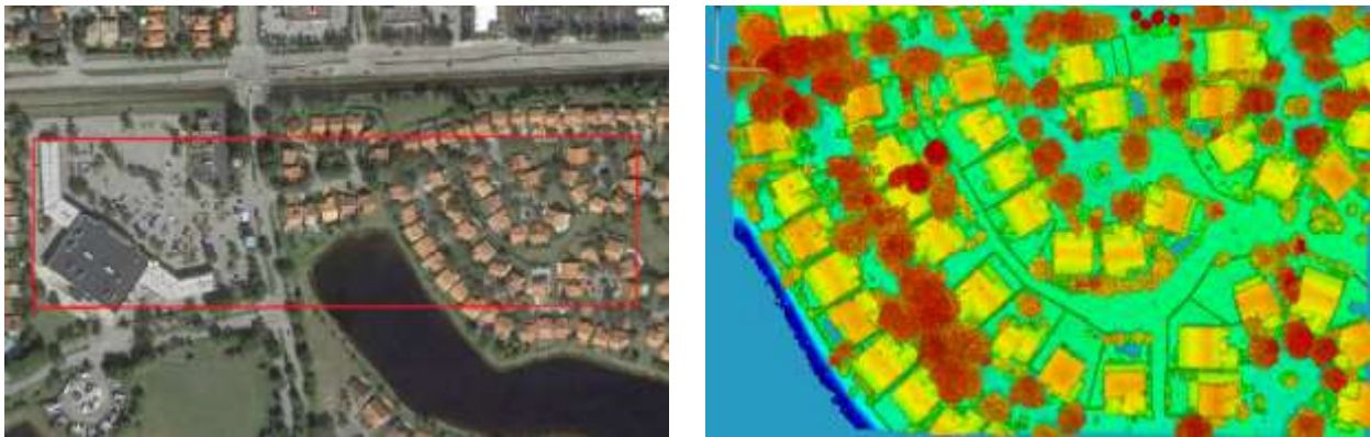
Figure 5-13: (Left) Study Area in USA; and (Right) Geiger Mode Lidar point cloud
