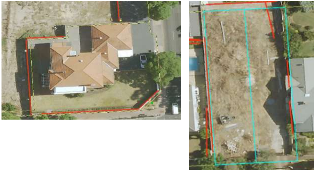
Figure 5-16: DCDB metadata states high accuracy but Lidar fence-lines match imagery not DCDB
