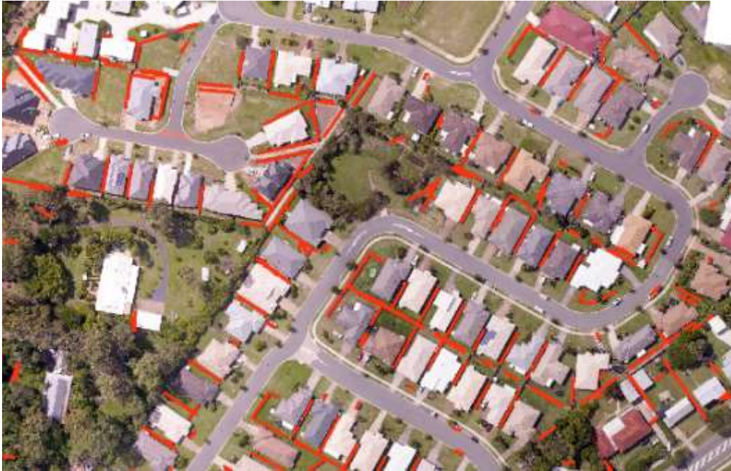
Figure 5-24: Fence-lines extracted from medium resolution Lidar for (Top) Horizontal and (Middle) Vertical directions of flight; and (Bottom) the combined Lidar results
