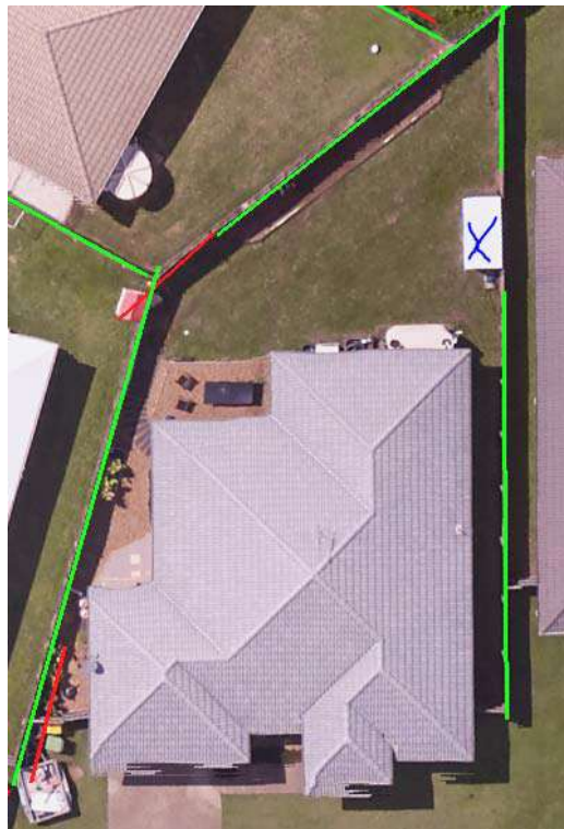
Figure 6-2: Small building/shed (blue X) is causing a section of the fence to be missed
