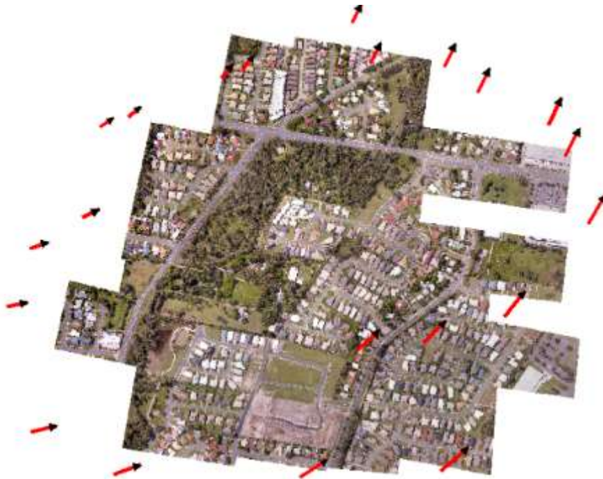
Figure 5-19: Link lines between extracted fence-lines and distorted cadastre for rubber-sheeting
