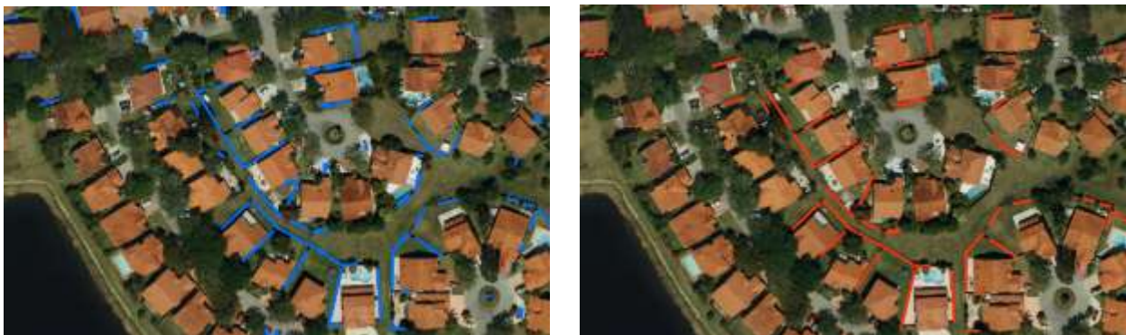
Figure 5-14: (Left) Unfiltered fence-lines and (Right) Filtered fence-lines extracted from Geiger Mode Lidar
