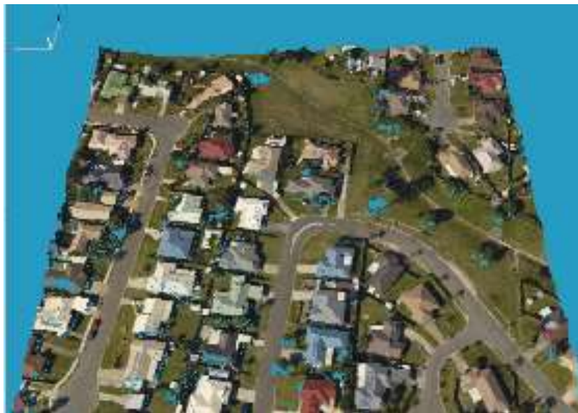
Figure 4-10: Dense point cloud generated from stereo-pair images by image matching
