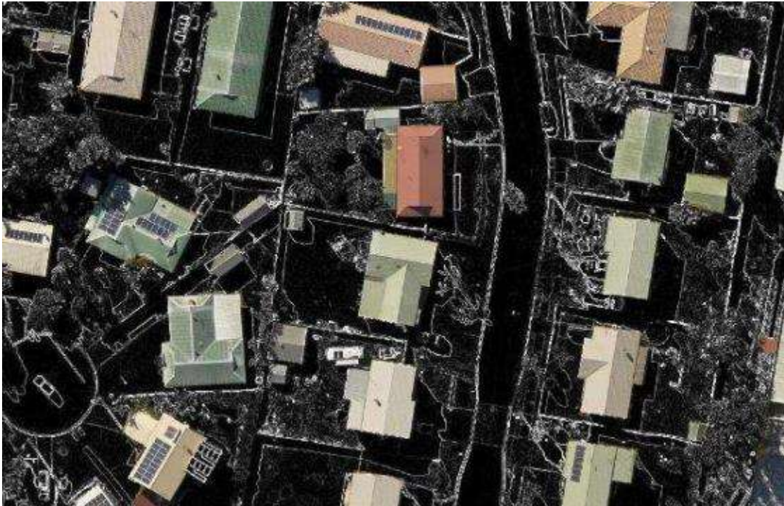
Figure 4-9: (Top) Edge detection shows a large number of edges; and (Bottom) Buildings overlaid on the edges
