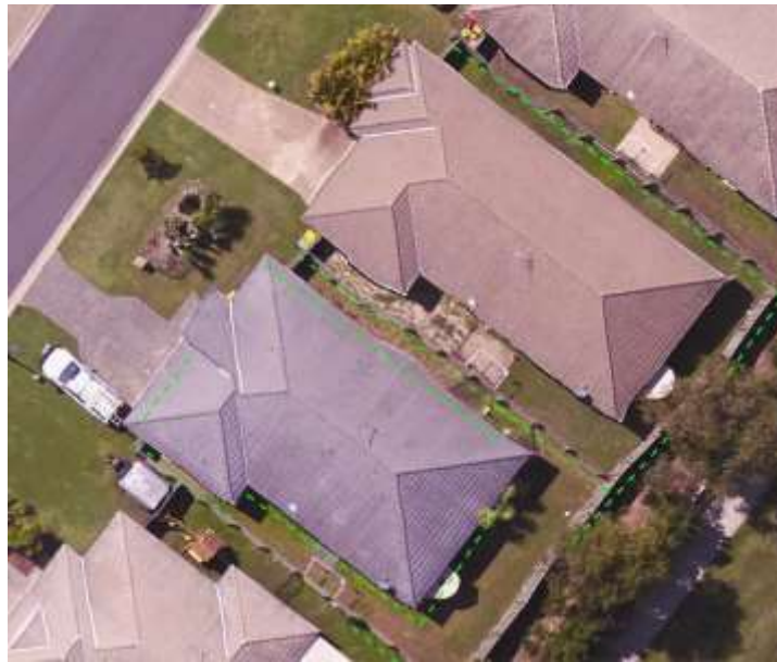
Figure 6-7: An example of the sides of a building being misclassified as a fence line (not common in Lidar extraction but very common in image-based extraction)
