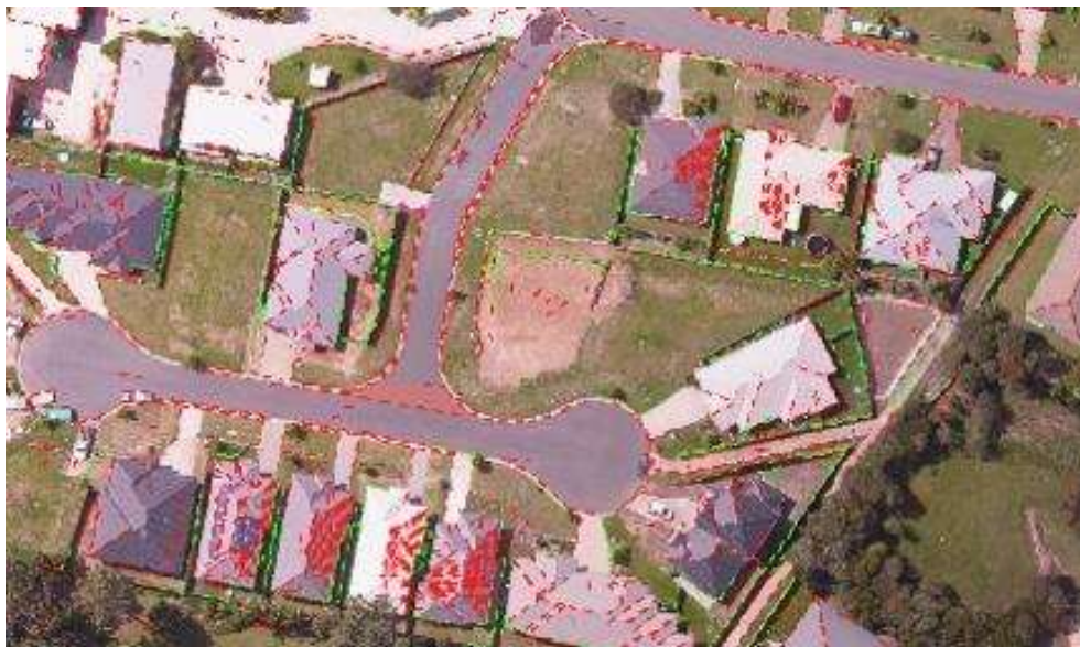
Figure 5-6: SVM filtering results in lines in green to be selected as fences, and lines in red are rejected
