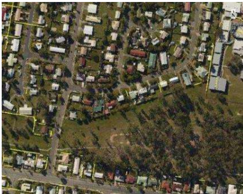
Figure 4-5: Fences detected using powerline algorithm showing false positives and omissions
