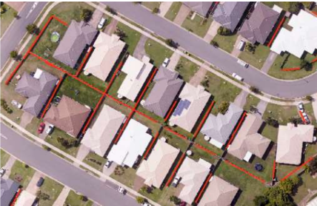
Figure 3-5: Image capture and processing (Top) Aerial photo of 6cm GSD; (Middle) Systematic shift noticed during ortho-rectification; (Bottom) Ortho-rectified imagery using GPS ground control
