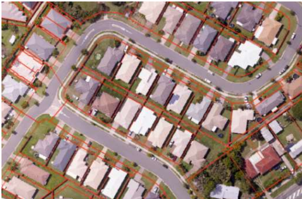
Figure 5-21: The DCDB was able to be block adjusted to its original high accurate position using the extracted fence-lines
