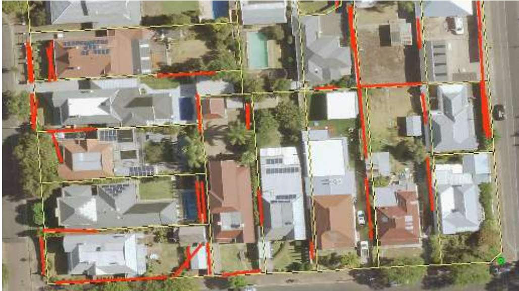
Figure 5-17: DCDB metadata states low accuracy, still Lidar fence-line extract matches imagery not DCDB
