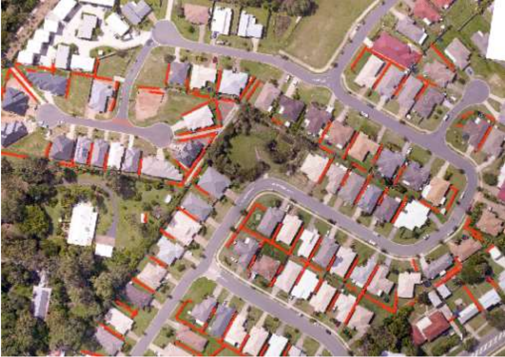
Figure 5-23: Fence-line extraction from high-resolution extraction shows a large percentage of visible fence-lines extracted
