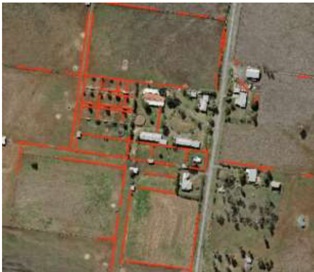
Fence-lines after SVM filtering
